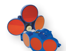
Workhorse Horizontal ADCP that “looks out” horizontally from its mounting structure to measure near-surface water currents and multi-directional waves.
